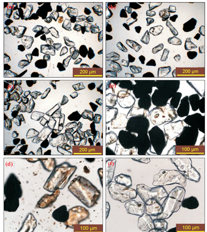
Fig. 9. Photomicrographs of heavy minerals in silica sand deposits: (a - c) heavy mineral assemblage under low magnification, (d - f) heavy mineral assemblage under high magnification. In high magnification photomicrographs the dark-coloured opaque minerals are mainly ilmenite and the light elongated transparent minerals are sillimanite.
