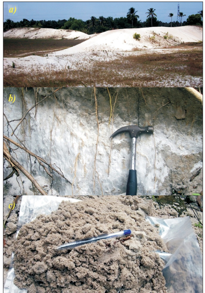
Fig.3. Field photographs showing a) A distant view of Silica sand dune deposits of Cherthala; b) Vertical section of the silica sand deposit; c) Silica sample collected for analysis
