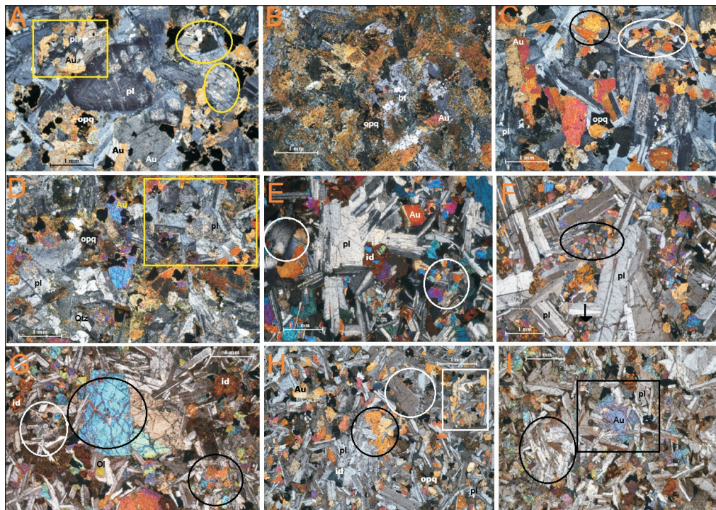
Fig.4. Photomicrographs of dolerite dykes (CD-1 to CD-9) under BXP and PPL (4×), (A) CD-1: Zoned plagioclase with porphyritic and sub-ophitic textures; sericitization noted, (B) CD-2: Chlorite and biotite showing weathered, dusty appearance, (C) CD-3: Augite with Carlsbad and penetration twins; symplectic and intergranular textures, (D) CD-4: Plagioclase altering to sericite with minor quartz; symplectic texture, (E) CD-5: Glomeroporphyritic and sub-ophitic textures; undulose extinction; olivine altered to iddingsite, (F) CD-6: Intersertal, intergranular, and nesophitic textures; coalesced plagioclase grains, (G) CD-7: Poikilitic texture with intersertal groundmass, (H) CD-8: Glassy micro-vein and nesophitic texture and (I) CD-9: Plagioclase laths penetrating augite; intersertal texture. Abbreviations: Pl–Plagioclase, Au–Augite, Opq–Opaque, Id–Iddingsite, Qtz–Quartz, Bt–Biotite, Chl–Chlorite.
